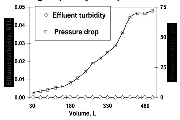
A 2.5" diameter X 5" pleated cartridge was challenged by 250 NTU of A2FTD @ 1.5 gallons/min. At 90 minutes (141 gallons) it had filtered out 119 grams of dust while producing an effluent < 0.01 NTU, at which point the test was terminated because of excessive pressure drop, but without breakthrough. It had removed >99.996% of dirt throughout the test.
