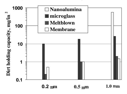
It's dirt holding capacity of 574 mg/in<sup>2</sup> is almost twenty times greater than microglass filter media when compared at a pore size rating of 1 µm and far greater than that if compared at the smaller pore size ratings.
