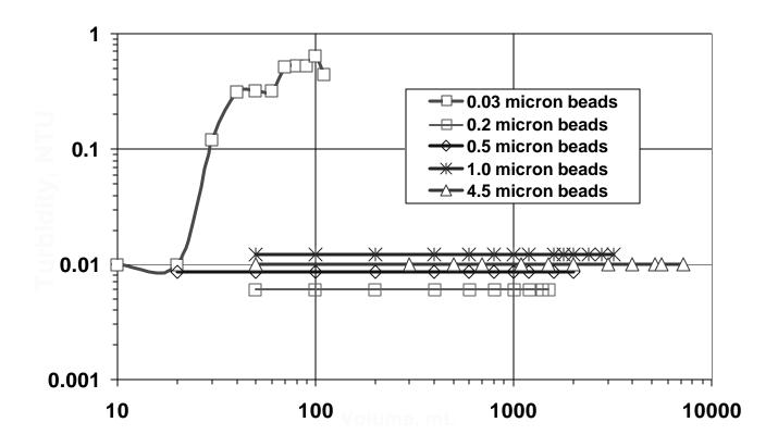
When a single layer of filter 25 mm in diameter was challenged by a continuous stream of latex beads it will eventually clog without exhibiting breakthrough, except with the smallest (0.03  $\mu$ m) beads. Bacteria size particles (0.2 to 4.5  $\mu$ m) are intercepted with high efficiency. A small virus would require a thicker filter in order to achieve 4 LRV.
