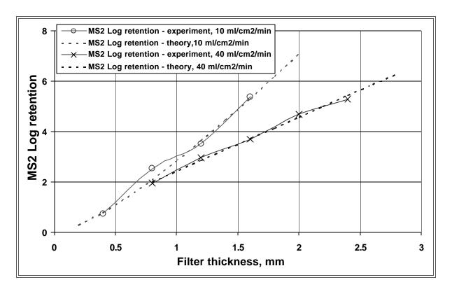
The model was tested with MS2 virus (25  $\mu$ m). This figure shows projected retention as a function of filter thickness for two different flow velocities. Experimental data show a high correlation with the model. Note that virus retention is predictable to at least 6 LRV.
