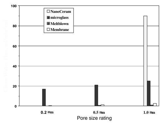
This shows NanoCeram's flowrate, superimposed over Shields' data [1] for clean water flow of several types of filter media. The nominal pore size of NanoCeram is 2-3 µm average, providing a major benefit in flow vs. 1.0 µm pore size of all other medias. If compared at smaller pore sizes, the flow benefit of NanoCeram would be huge. Yet NanoCeram has higher filtration efficiency when compared to any of the others, irrespective of pore size rating.
