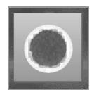
When the ink was injected through the NanoCeram® filter, the back pressure was low and filtration was easy. Yet the effluent came out water white. The filter (above) was intensely colored, proving that it retained nanometer size particles while the 25 nm UP membrane was ineffective.
