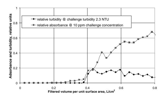
The filter is excellent for adsorbing turbidity. Filters (25 mm diameter) were challenged with humic acid, an organic particle small enough to pass through "Absolute"  $0.2~\mu$  filters. Breakthrough was detected by both optical turbidity and spectrophotometric methods. Note the high filtration efficiency until the filter is exhausted at about 0.4~L of fluid/cm<sup>2</sup> of filter area.
