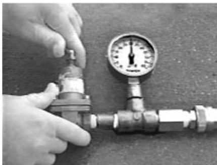
**Figure 14-5 Pressure Adjustment**
